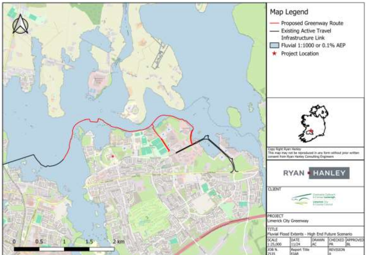
Figure 8-15 High End future flood risk, low probability (i.e. 0.1% AEP) event flood extents
